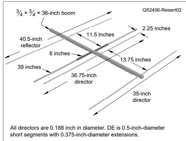
Figure 2 — Dimensions of the 2-meter Yagi.
